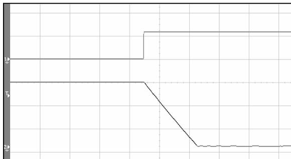
Figure 8 Output voltage shutdown by remote OFF, (2ms/div), see Figure 10 for test configuration; CH1-remote OFF voltage (5V/div); CH2-output voltage (10V/div)
